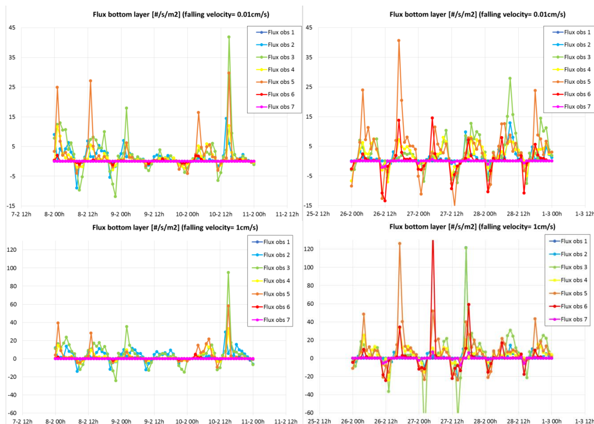
Figure 5.17 Near bed particle fluxes (current velocity * concentration) at cross-sectional observation locations for falling particles for different falling velocities and periods
