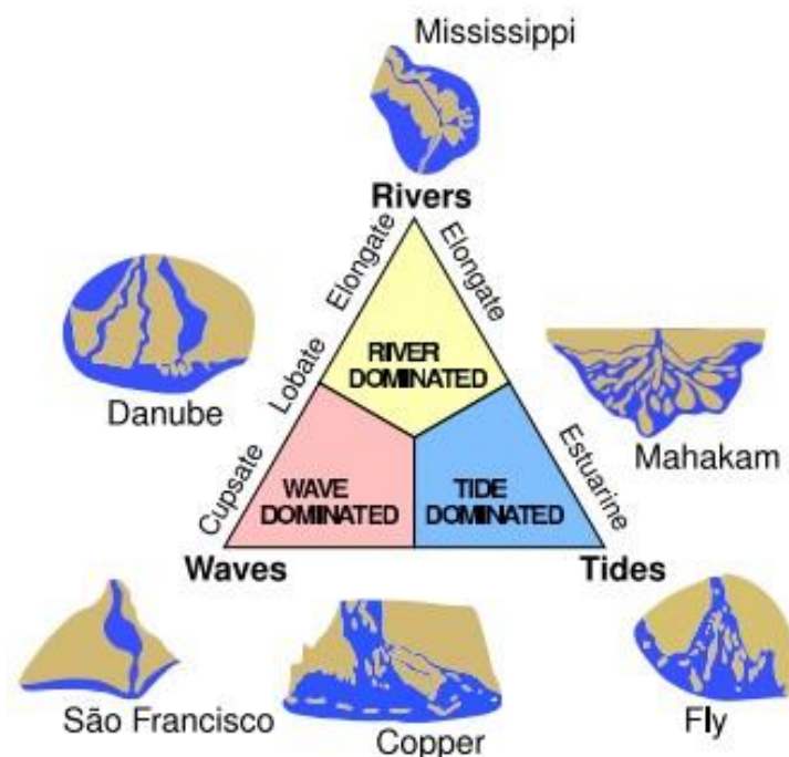
Figure 2.10 Classification of deltas by the forcing dominant in forming the delta (Seybold et al. 2007)
