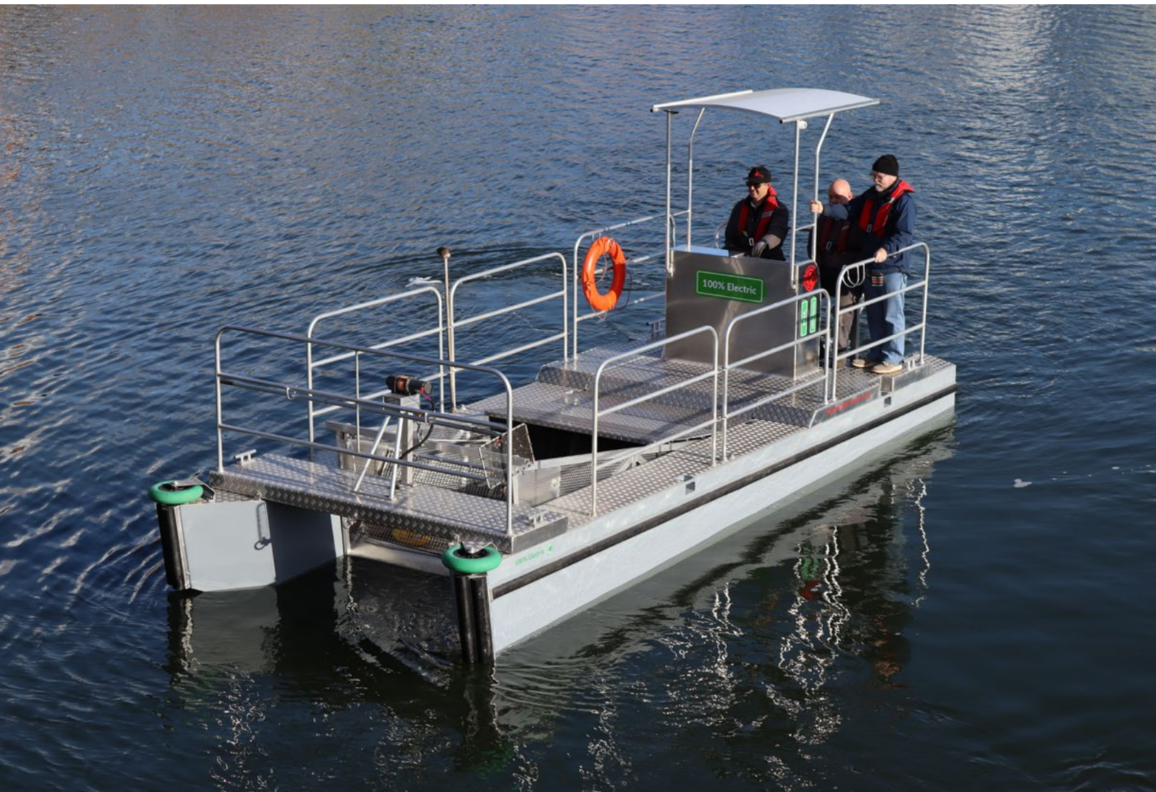
The Versi-Cat Trash Skimmer Boat by Water Witch collects floating and semi-submerged litter, debris and aquatic vegetation from the water surface into a removable basket, which can be lifted and tipped directly into a skip or shore side receptacle for disposal. Credit: Water Witch
