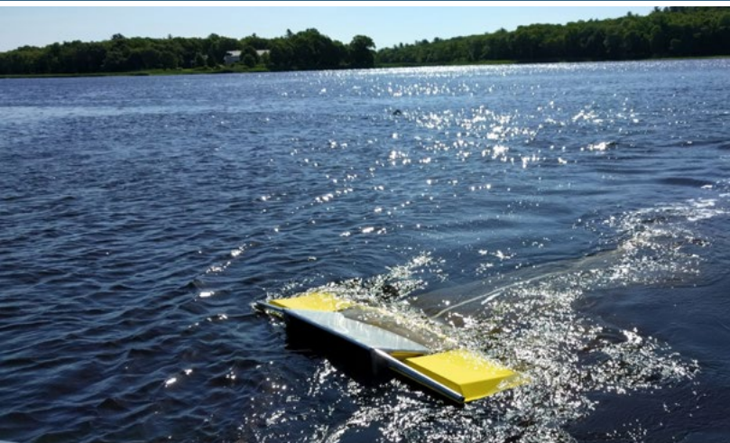
The Manta Trawl allows Save The Bay's Waterkeepers to collect microplastics from surface water in Narragansett Bay. Credit: Save the Bay - Narragansett Bay
