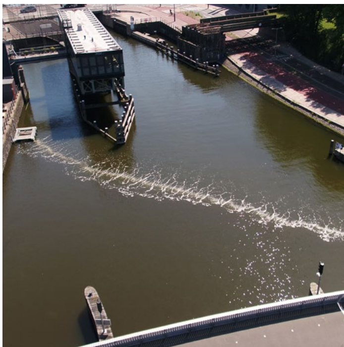
The Bubble Barrier in Westerdok Canal, Amsterdam. Credit: The Great Bubble Barrier
