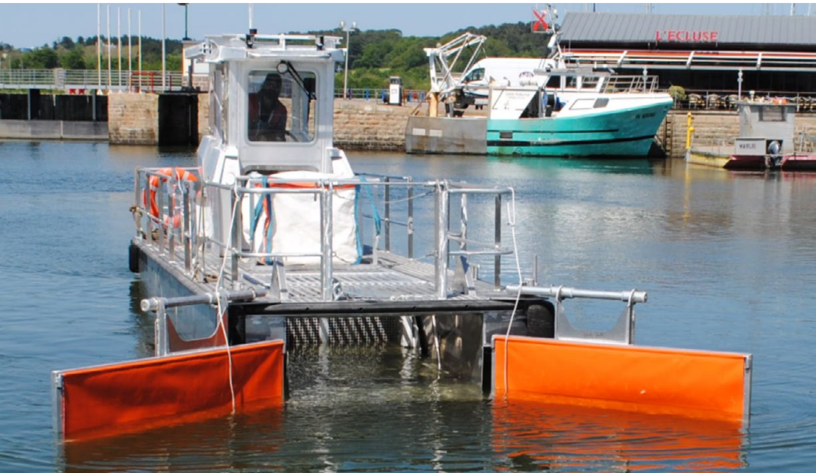
The WasteCleaner 92 by Efinor collects solid and liquid waste, with a capacity of 1200kg for solid waste such as plastics and 4000L for liquid waste such as oil. Credit: Efinor
