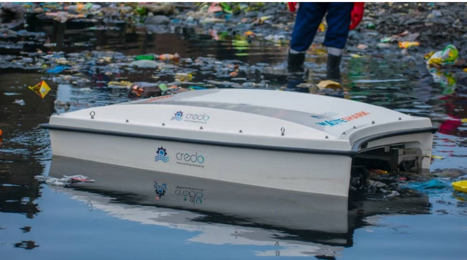
The WasteShark by RanMarine is an autonomous surface vessel that is modelled after the whale shark and produces zero greenhouse gas emissions. Credit: RanMarine
