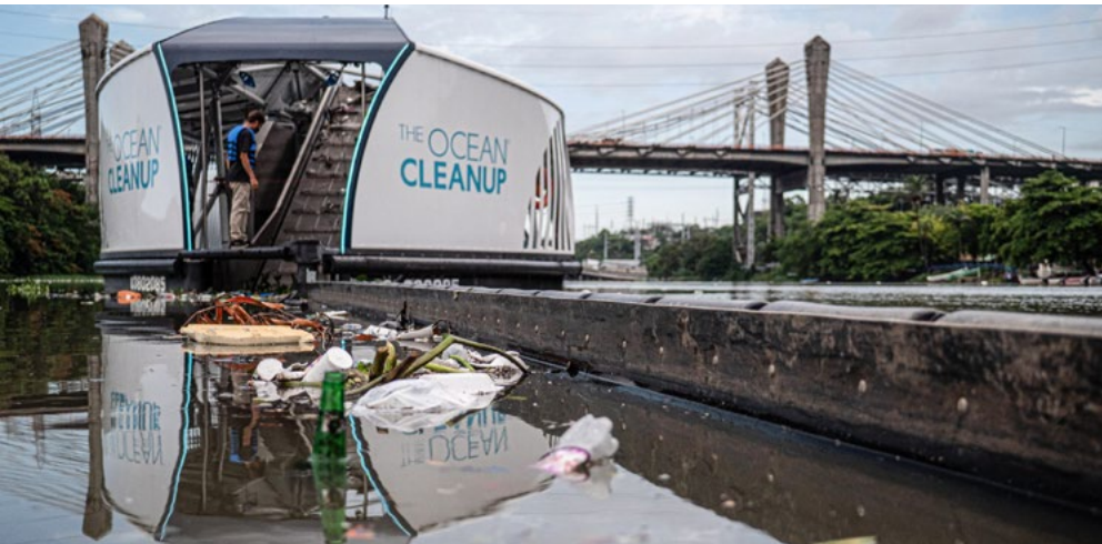
The Interceptor™ uses a solid barrier to catch and concentrate debris towards a conveyor belt fitted onto a floating pontoon. Santo Domingo, Dominican Republic. Credit: The Ocean Cleanup
