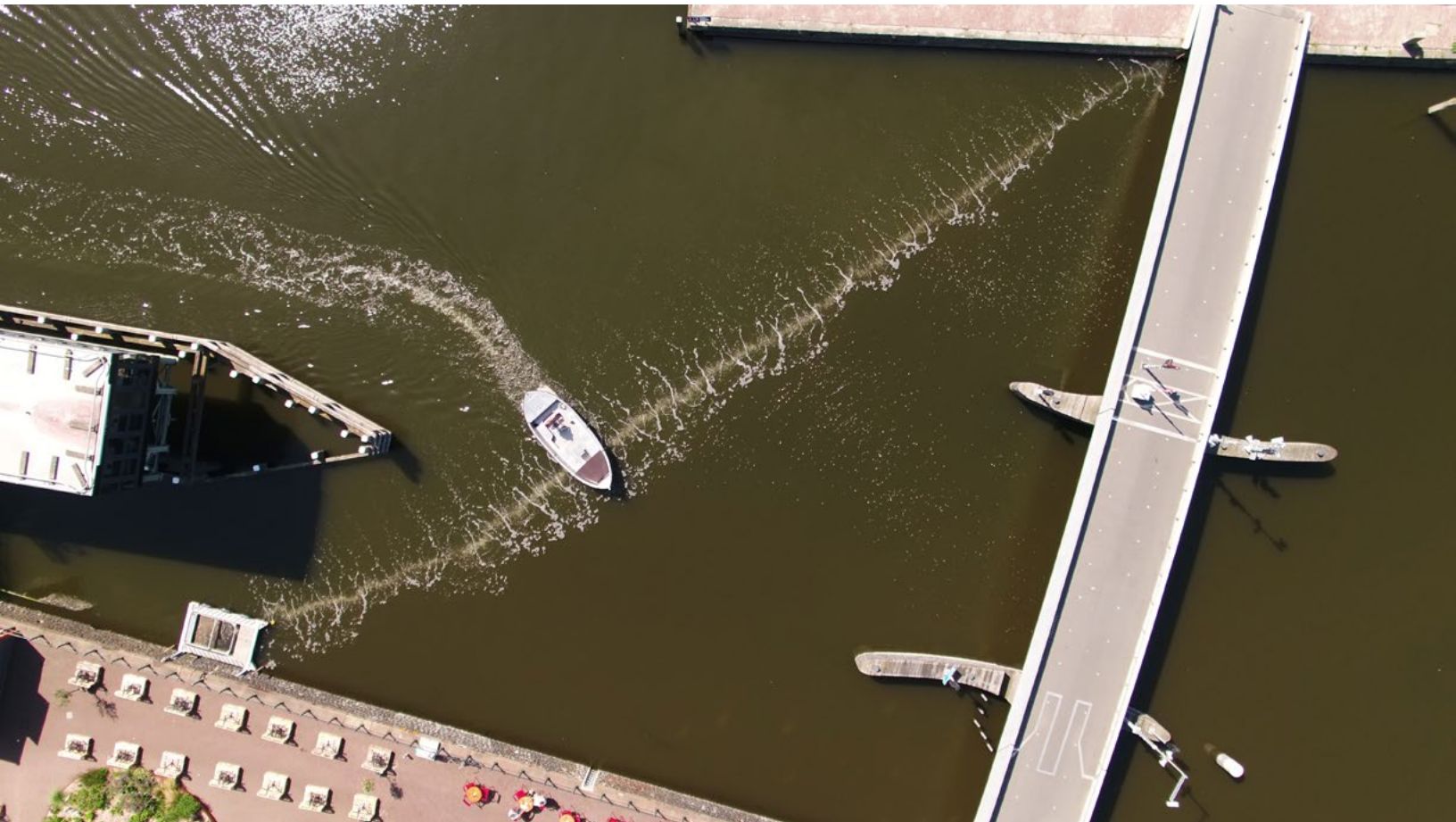
The Bubble Barrier creates a barrier to stop plastics from flowing past, while allowing fish and ships to pass through unimpeded. Westerdok Canal, Amsterdam, the Netherlands. Credit: The Great Bubble Barrier
