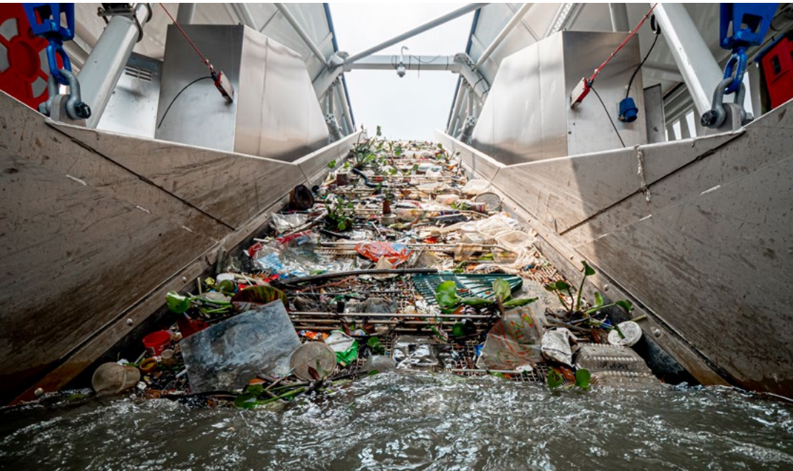
The conveyor belt of Interceptor 002™ in Klang River, Malaysia. Credit: The Ocean Cleanup
