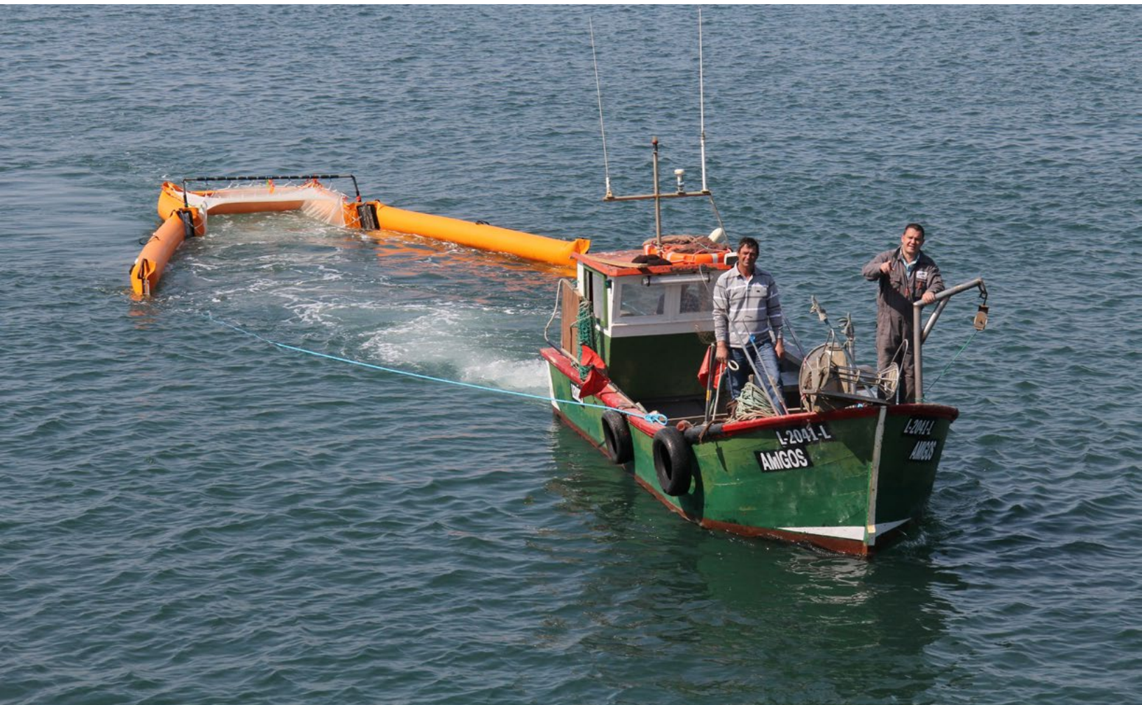
The Trash Catcher by Waste Free Oceans is designed to be towed by a fishing vessel. Credit: Waste Free Oceans
