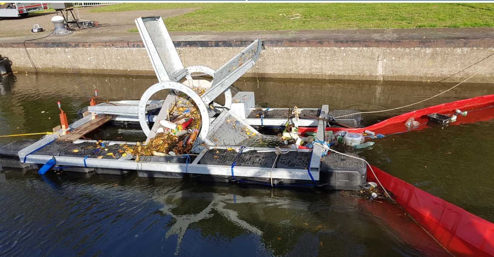
The CirCleaner by Noria Sustainable Innovators in Rotterdam, the Netherlands, funnels plastic debris into the trap where it is lifted out of the water with a small water wheel. Credit: Noria Sustainable Innovators
