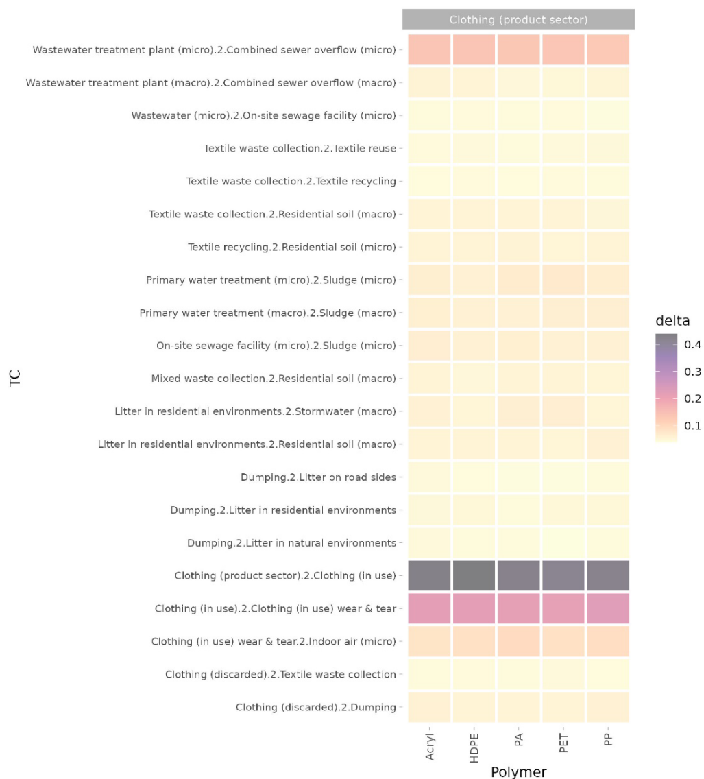
Figure D17 Sobol Indices for Clothing textiles from global sensitivity analysis of input variation in transfer coefficients in relation to output variation of plastics emitted to the environment.
