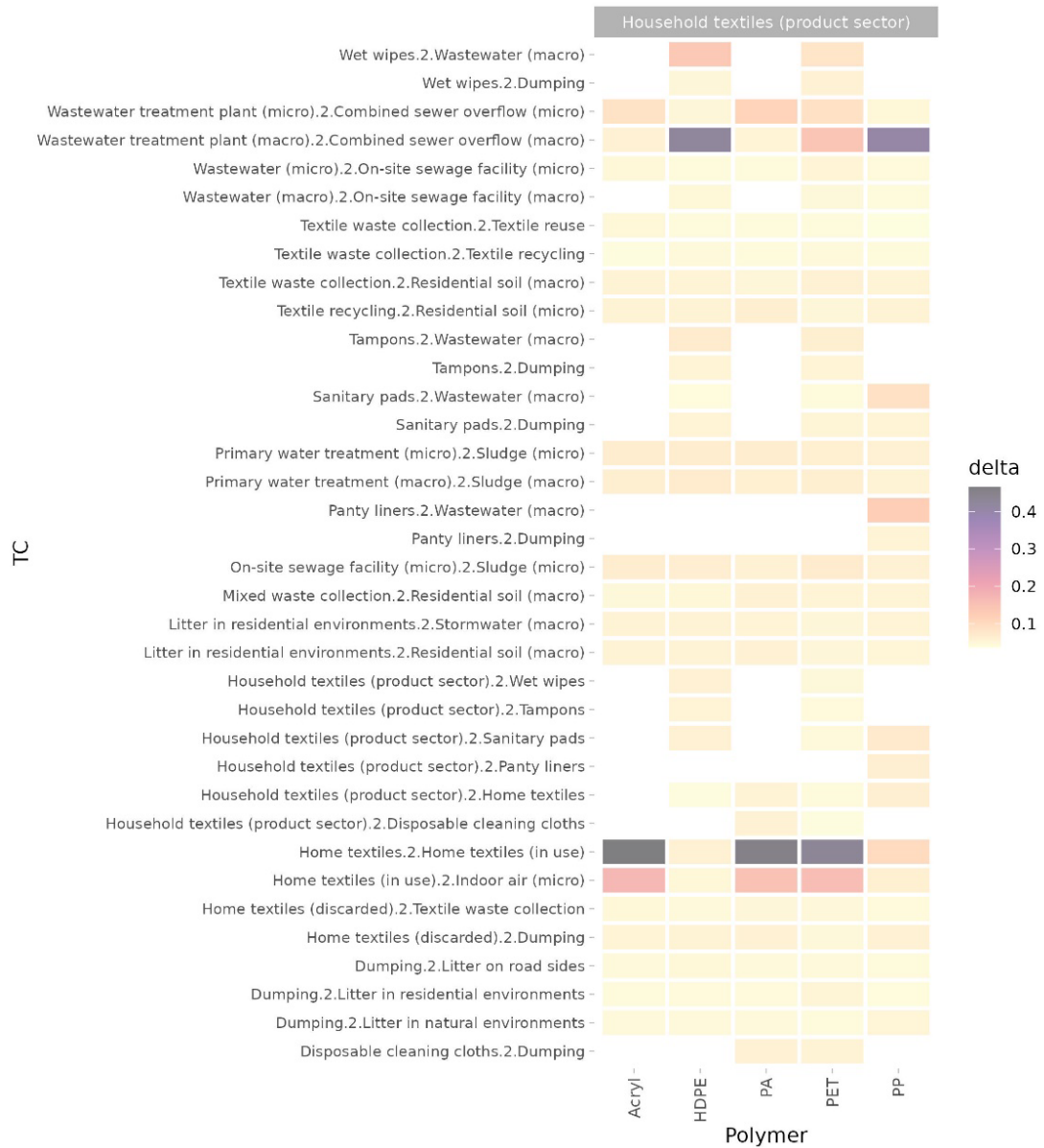
Figure D15 Sobol Indices for Household textiles from global sensitivity analysis of input variation in transfer coefficients in relation to output variation of plastics emitted to the environment.
